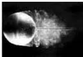
2. Laminar separation behind a sphere
