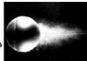
3. Turbulent separation behind a sphere
