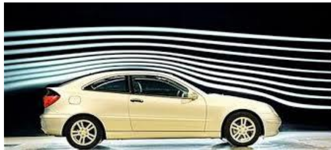
Figure 3.5 Smoke path/streak/streamlines in steady flow over an automobile.
