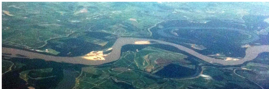
Figure 7.8 An image of river meandering, clearly showing sand bars (appearing as light yellow) formed on the inside of bends (curves) in the river.
