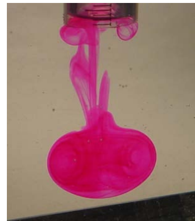
Figure 1: Vortex ring in water formed with rhodamine dye.
