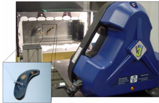
Fig. 1: The simulated fish in the water channel showing the location of the V3V camera. (Inset: close view of the model).
